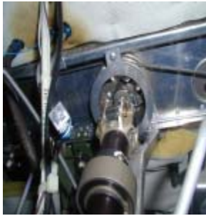
Forward end of the control yoke assembly and the box bearings installed over the control tube assembly at the aileron drum.
