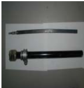
The result of too much force, improper directional load and, of course, LACK OF LUBRICATION!
